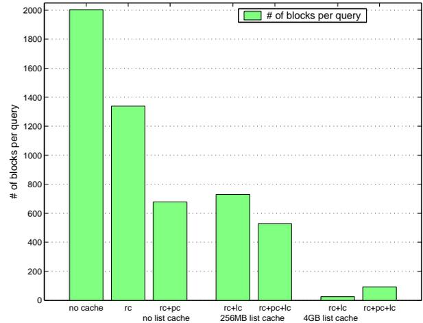
**Figure 6.7: Number of block reads per query, for the following seven schemes (from left to right): no caching, result caching, result plus projection caching, result plus list caching and all three levels of caching with a 256 MB list cache, and result plus list caching and all three levels of caching with a 4 GB list cache.**
