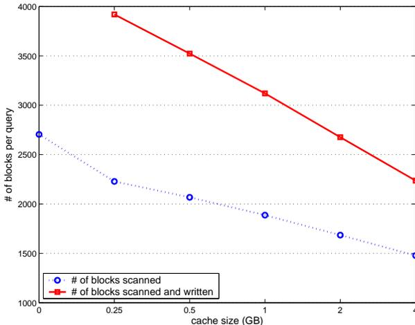
**Figure 6.4: Block reads (lower graph) and block reads plus writes (upper graph) per executed query, without projection caching and with different amounts of cache space under the basic *Landlord* approach.**
