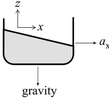
The body force per unit volume that acts on an element in the accelerating fluid has the form  $\mathbf{F}_v = -\rho a_x \delta_x - \rho g \delta_z$ , where the force component along the  $x$  direction,  $F_{vx}$ , is equal to  $-\rho a_x$  (note that when the container of fluid is accelerated in the  $+x$  direction, the fluid element experiences an inertial body force that acts in the  $-x$  direction). Equations (3) become
