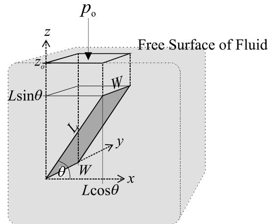
The total body force on this fluid volume due to gravity is (the minus sign indicates that the force acts in the  $-z$  direction):
