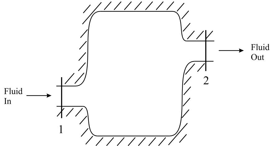
Designating the entry port as port "1" and the exit port as port "2", we want to sum equation 9 for all streamlines passing through these ports. The contribution of each streamline to the sum must be weighed by the rate at which fluid mass passes along it through the control volume. This rate of mass flow is  $\rho \mathbf{v} \cdot \mathbf{n}$ , where  $\mathbf{n}$  is the unit normal to the surface of the control volume.
