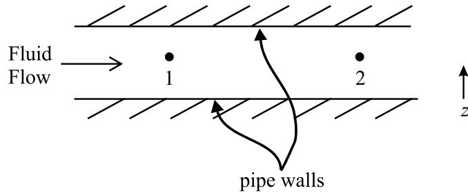
If the flow is steady and incompressible, and  $z_1 = z_2$ ,  $v_1 = v_2$ , and  $w_s = 0$ , then equation 9 becomes:
