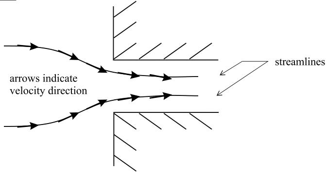
**Path Lines:** lines traced out by fluid particles moving with the flow. At steady state, streamlines and path lines are equal.
