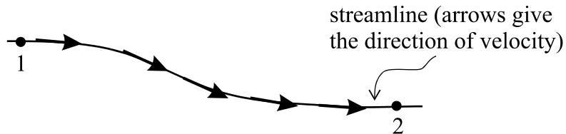
Along the streamline,  $\mathbf{ds}$  is used to represent a differential displacement:
