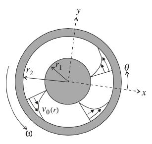
c). How could you use this device to measure viscosity?
