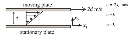
The flow is steady, incompressible, and laminar.
