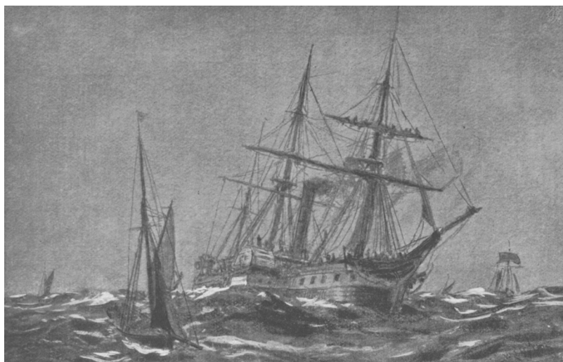
FIG. 5 The Acadia (1840), built by John Wood as the “pattern card” for the first four Cunarders and using Robert Napier’s 420-horsepower side-lever engines. (Source: James Napier, Life of Robert Napier of West Shandon [Edinburgh, 1904].)
