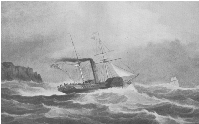
FIG. 1 Portrait of the 350-ton paddle steamer Isabella Napier (1835), fitted with 220-horsepower side-level engines, defying the strong onshore wind and sea dreaded by sailing vessels and fighting its way from the Clyde to Londonderry in the service of the North-West of Ireland Steam Packet Company. (Source: James Napier, Life of Robert Napier of West Shandon [Edinburgh, 1904].)
