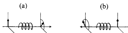
FIG. 3.23. Rotation of the plane of polarization of light traveling through a helix for two opposite directions of propagation.
