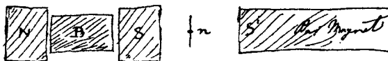
FIG. 3.11. Faraday's replication of Weber's experiment for testing the magnetic polarization of a bismuth block (B) in the field of a horse-shoe magnet (NS), with a compass needle n and a compensatory bar-magnet S' (FD 5: 153).
