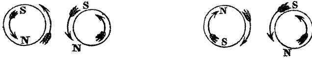
FIG. 1.8. Wollaston's diagram for the attraction of two parallel currents (left) and the repulsion of antiparallel ones (right).
