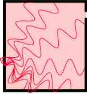
The higher the frequency, the more modes you can fit into the cavity.*
