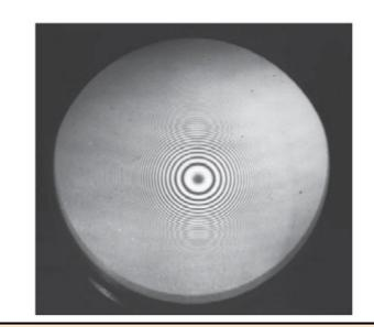
Air film between a convex lens and a plane surface. The thickness of the film t increases as we move out from the center, giving a series of alternating dark and bright rings.
