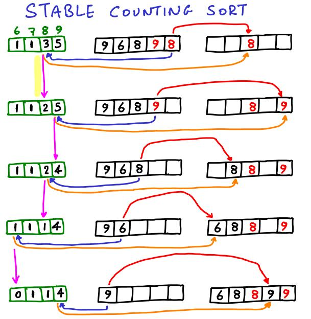
the first time we point to the count array at index i... ... it tells us where the <u>last</u> element with value i must go 1135 Then we decrement so the next element with value i (to the left in input array) will have its correct empty place.
