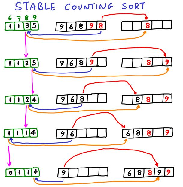
the first time we point to the count array at index i... ... it tells us where the <u>last</u> element with value i must go 1135 Then we decrement so the next element with value i (to the left in input array) will have its correct empty place. We will only decrement once per element with value i
