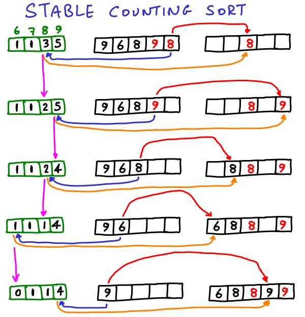
the first time we point to the count array at index i... ... it tells us where the <u>last</u> element with value i must go 1 1 3 5 Then we decrement so the next element with value i (to the left in input array) will have its correct empty place. We will only decrement once per element with value i, so we maintain # in index i > max # in index i-1 no conflicts
