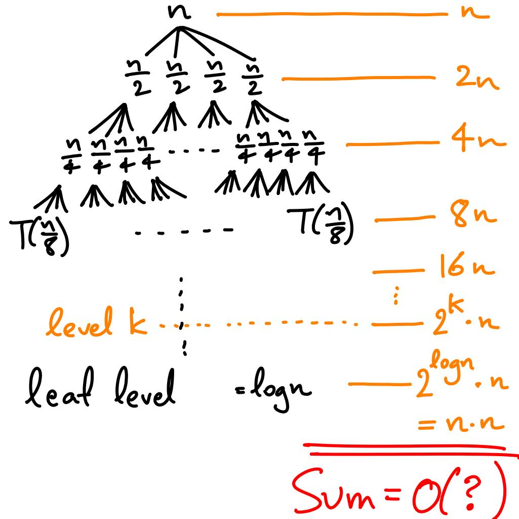
$$T(n) = 4T\left(\frac{n}{2}\right) + n \quad \text{by recursion tree}$$
