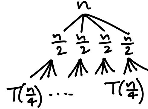
$$T(n) = 4T\left(\frac{n}{2}\right) + n \quad \text{by recursion tree}$$
