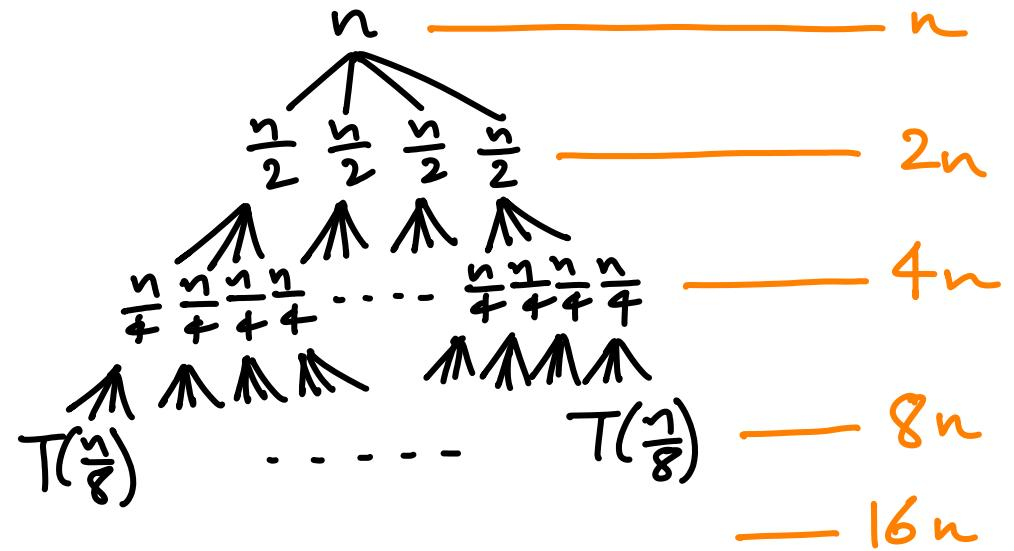
$$T(n) = 4T\left(\frac{n}{2}\right) + n \quad \text{by recursion tree}$$
