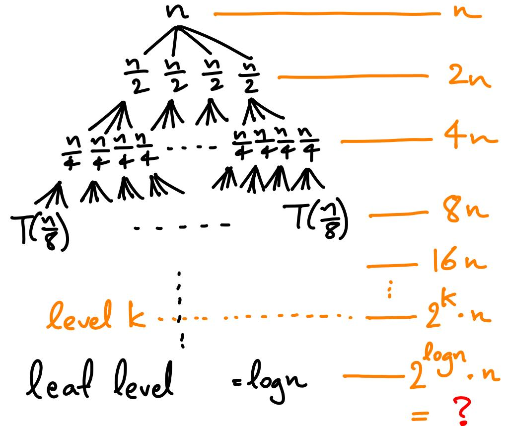
$$T(n) = 4T\left(\frac{n}{2}\right) + n \quad \text{by recursion tree}$$
