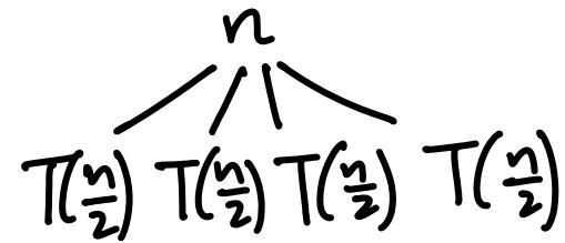
$$T(n) = 4T\left(\frac{n}{2}\right) + n \quad \text{by recursion tree}$$
