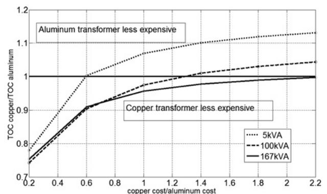
**Figure 6** Ratio of TOC (\$) of copper transformers over TOC (\$) of aluminium transformers as a function of the ratio of copper unit cost (\$/kg) over aluminium cost (\$/kg) for 5, 100 and 167 kVA single-phase transformers
