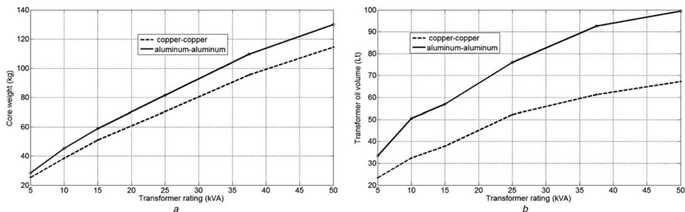
**Figure 7** Comparison of core weight and oil volume of copper versus aluminium transformers
