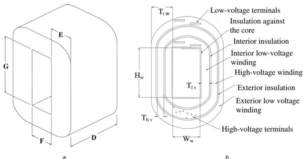
**Figure 8** Active part of single-phase shell-type transformer
