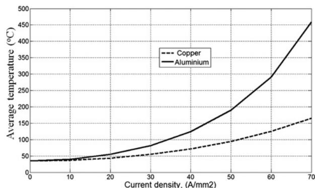
**Figure 4** Average temperature against current density for copper and aluminium under a short-circuit condition with duration of 4 s
