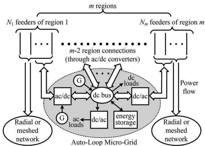
Fig. 2. Configuration of the auto-loop microgrid.
