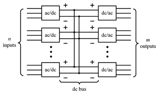
Fig. 3. Systematic structure of the dc link.
