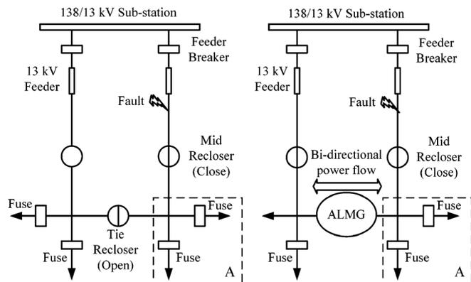
Fig. 1. Operation of auto-loops. (a) Configuration of a typical auto-loop distribution system. (b) Configuration of an auto-loop microgrid.
