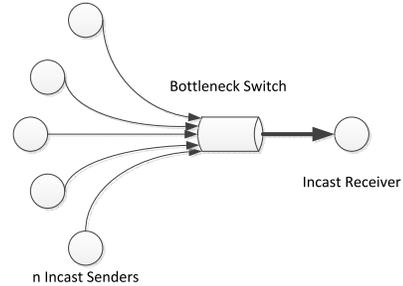
Fig. 1. Incast traffic is a high fan-in, many to one data transfer.
