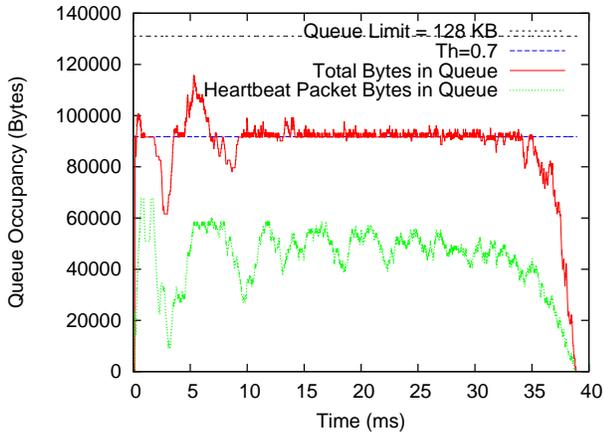
Fig. 22. Instantaneous queue occupancy for incast setting of 45 senders sharing a 128 KB bottleneck switch buffer. SRU is 100 KB
