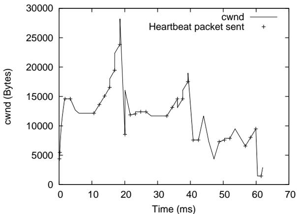
Fig. 24. Instantaneous cwnd for an incast sender. Time instants when a heartbeat packet is sent is indicated
