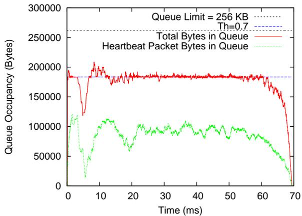
Fig. 23. Instantaneous queue occupancy for incast setting of 80 senders sharing a 256 KB bottleneck switch buffer. SRU is 100 KB
