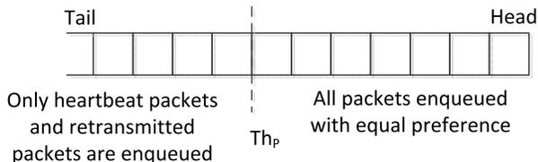
Fig. 10. Queuing mechanism for PLATO
