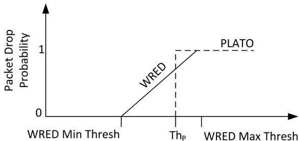
Fig. 9. WRED and PLATO drop probability for regular packets.
