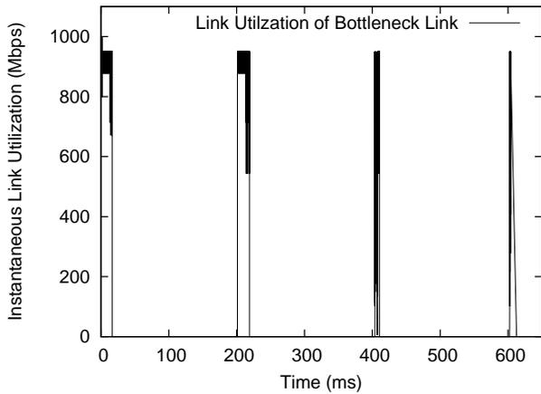
Fig. 2. Link utilization for the bottleneck link for 45 servers sending 100 KB SRU to 1 client over a 256 KB bottleneck switch buffer. All servers and client use TCP NewReno.
