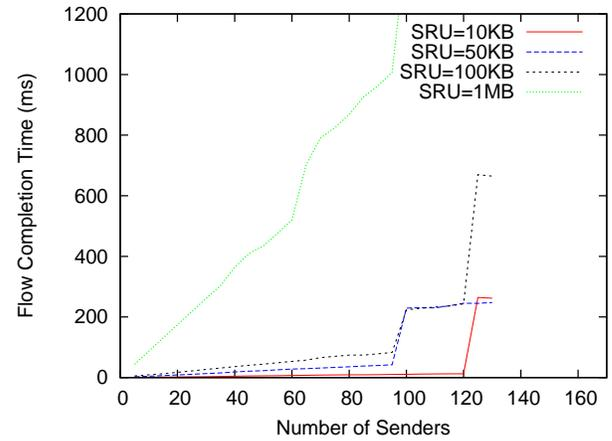
Fig. 14. Flow completion time, for PLATO flows. Switch buffer size is 256 KB and  $Th_P$  is 0.7
