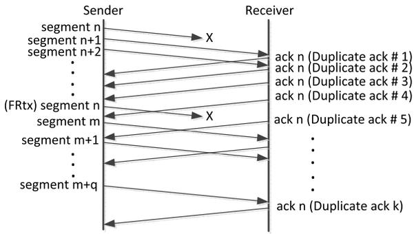
Fig. 5. Double Loss: Loss of retransmitted packet.
