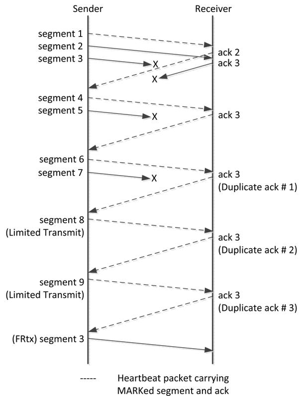
Fig. 6. A simplified implementation of PLATO. Limited Transmit [19] when enabled, allows TCP to send a segment each for the 1<sup>st</sup> and 2<sup>nd</sup> duplicate acks.
