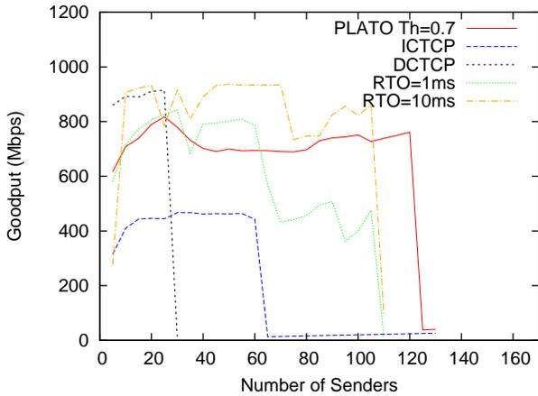
Fig. 19. Performance of PLATO compared to DCTCP, ICTCP and TCP NewReno with reduced  $RTO_{min}$  values of 10 ms and 1 ms. Switch buffer is 256 KB and SRU is 10 KB.  $Th_P$  is 0.7
