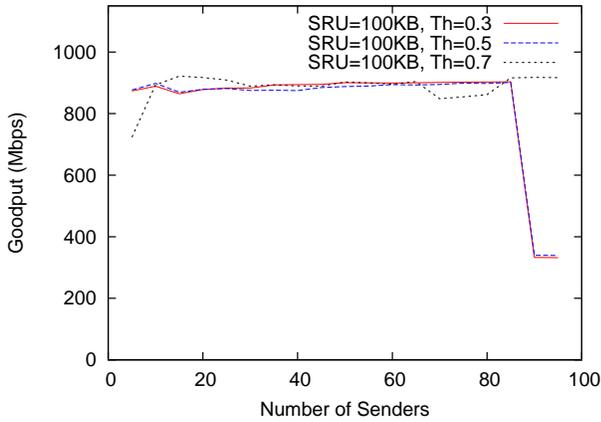
Fig. 12. Effect of  $Th_P$  on the performance of PLATO for long lived flows. Switch buffer is 256 KB and SRU is 100 KB
