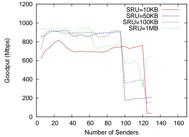
Fig. 13. Performance of PLATO for switch buffer size of 256 KB, under different SRU sizes.  $Th_P$  is 0.7
