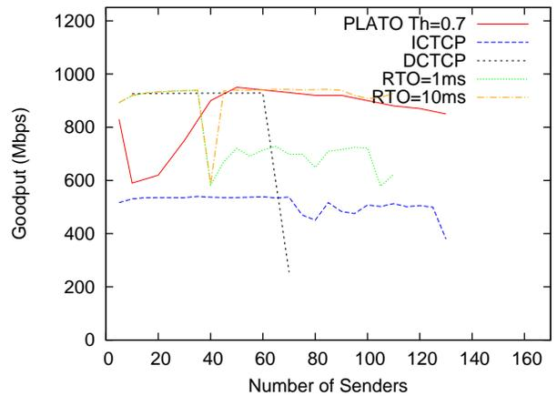
Fig. 21. Performance of PLATO compared to DCTCP, ICTCP and TCP NewReno with reduced  $RTO_{min}$  values of 10 ms and 1 ms. Switch buffer is 2 MB and SRU is 100 KB.  $Th_P$  is 0.7
