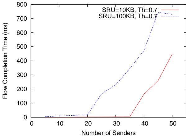
Fig. 16. Flow completion time, for PLATO flows. Switch buffer size is 64 KB and  $Th_P$  is 0.7
