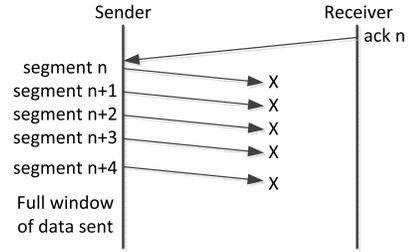
Fig. 3. Block Loss: All the segments from a window are lost.
