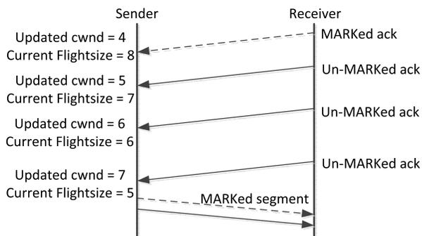
Fig. 8. Inability to send new data in response to labelled ack is not indication of stalled cwnd. Some in-flight acks may allow cwnd to send data later.
