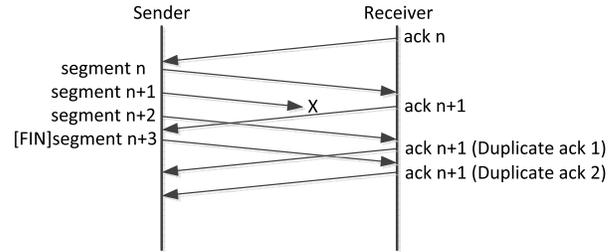
Fig. 4. Tail Loss: One of the last three segments are lost.
