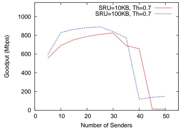
Fig. 17. Performance of PLATO with background TCP NewReno traffic. Switch buffer size is 256 KB.  $Th_P$  is 0.7
