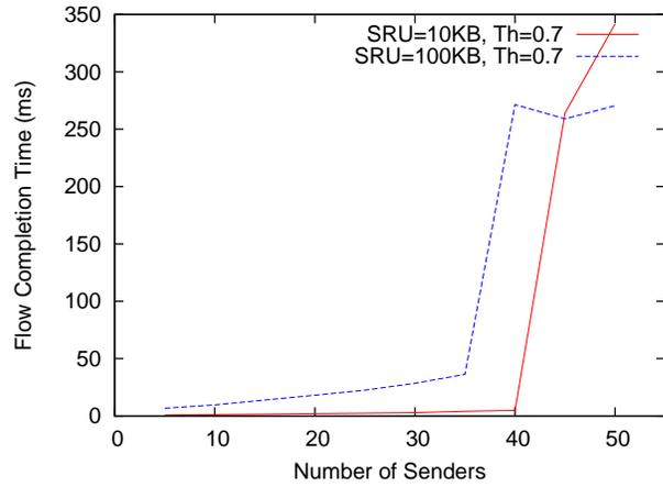
Fig. 18. Flow completion time, for PLATO flows, when background TCP NewReno flows are present. Switch buffer size is 256 KB and  $Th_P$  is 0.7
