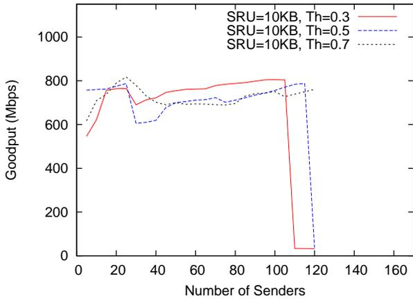
Fig. 11. Effect of  $Th_P$  on the performance of PLATO for short lived flows. Switch buffer is 256 KB and SRU is 10 KB
