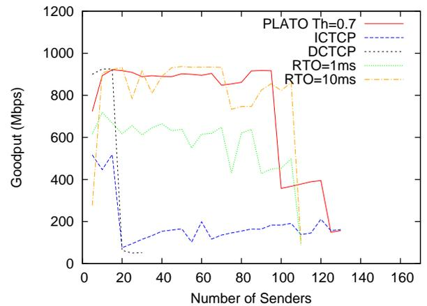
Fig. 20. Performance of PLATO compared to DCTCP, ICTCP and TCP NewReno with reduced  $RTO_{min}$  values of 10 ms and 1 ms. Switch buffer is 256 KB and SRU is 100 KB.  $Th_P$  is 0.7
