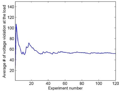
Fig. 9. Cumulative average of the number of loads with voltage violation (5%) as the number of experiments increases.
