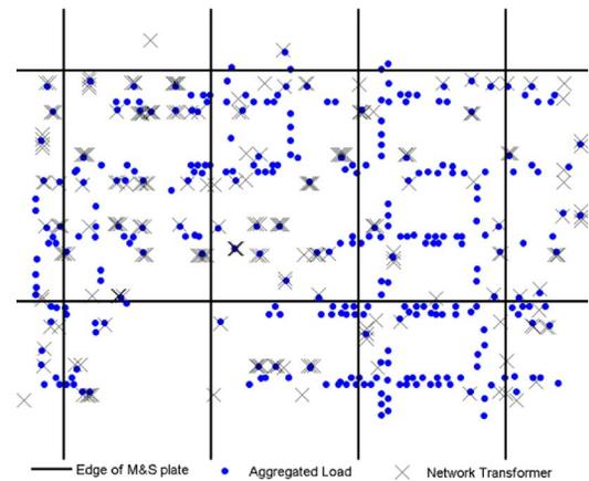
Fig. 3. Location of loads and transformers in the Sutton network using as reference the edges of the M&S plates.
