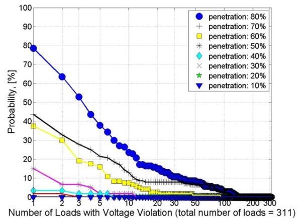
Fig. 8. Probability of having voltage violations of more than  $\pm 10\%$  versus the number of loads with violation.
