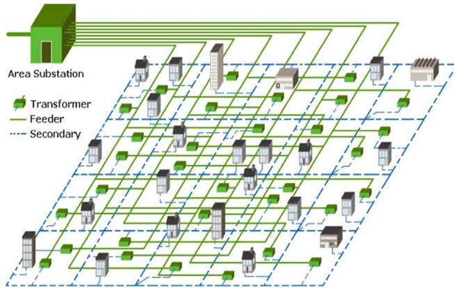
Fig. 1. Schematic of an LV secondary network. Loads and network transformers are tied together in a highly meshed network.
