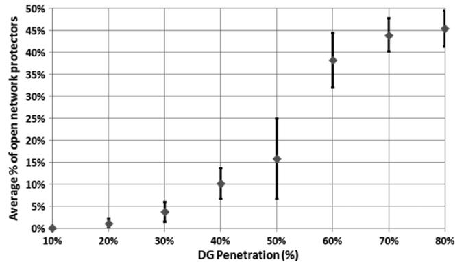
Fig. 11. Average percent of open network protectors versus the DG penetration level.
