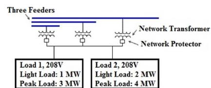
Fig. 4. Typical configuration of an isolated spot network.
