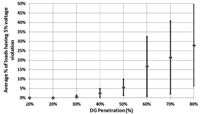
Fig. 10. Average percent of loads having voltage violations versus the DG penetration level.
