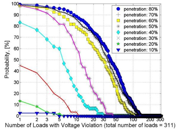
Fig. 7. Probability of having voltage violations of more than  $\pm 5\%$  versus the number of loads with violation.
