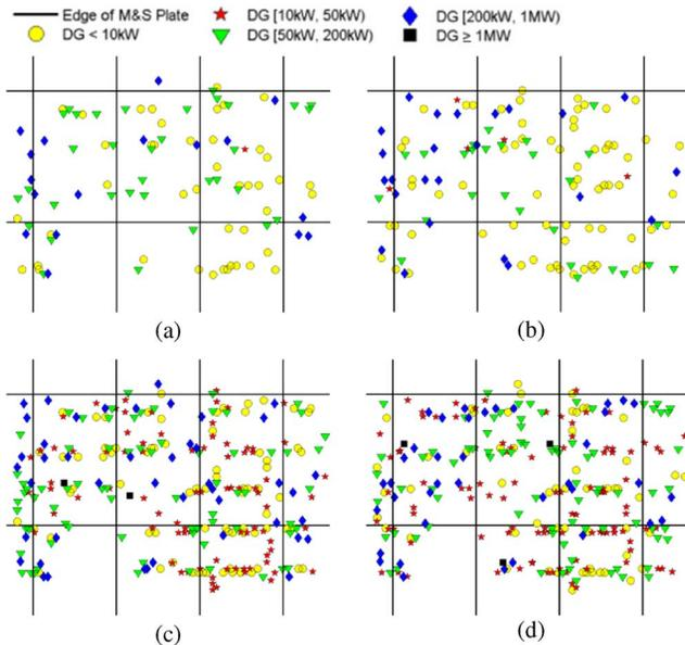
Fig. 6. Examples of DG allocation for different DG penetrations. (a) Case 1 at 20%. (b) Case 2 at 20%. (c) Case 1 at 60%. (d) Case 2 at 60%.
