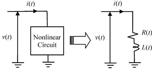
Fig. 3. Time-varying equivalent circuit with identical energy dissipation and storage characteristics.
