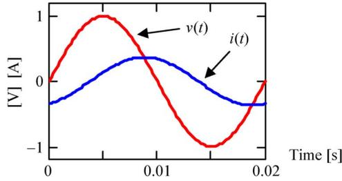
Fig. 4. Instantaneous current and voltage for a linear  $R$ - $L$  circuit.
