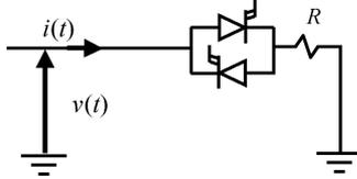
Fig. 8. Controlled rectifier feeding a resistive load.
