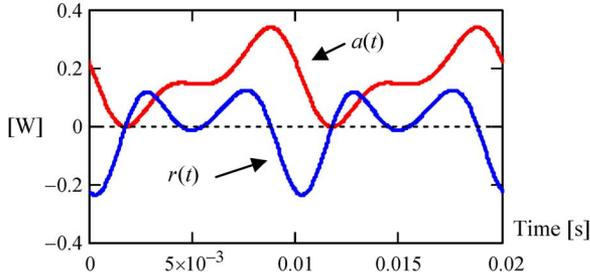
Fig. 25. Instantaneous active and reactive powers for the signals of Fig. 23.
