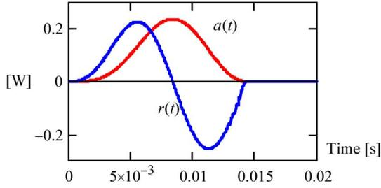
Fig. 14. Instantaneous active and reactive powers corresponding to the voltage and current signals of Fig. 12.
