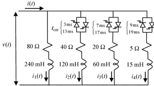
Fig. 15. Switching  $R$ - $L$  branches with the same time constant.
