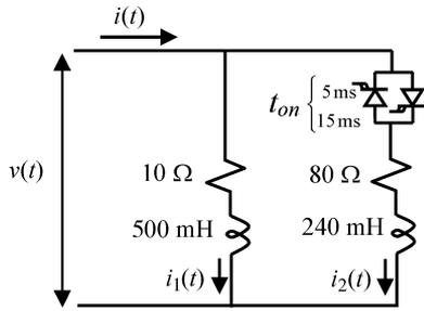
Fig. 19. Two parallel branches with different time constants.
