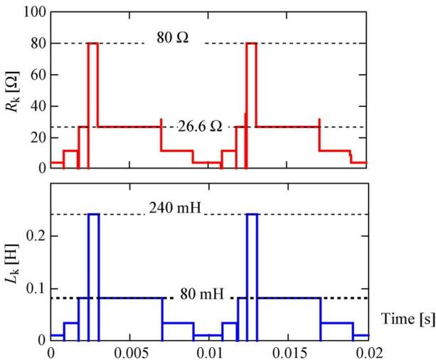
Fig. 17. Results of the identification process for the circuit of Fig. 15.
