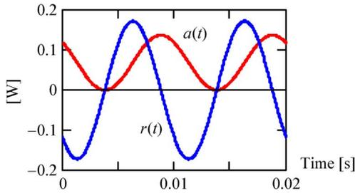
Fig. 6. Instantaneous active and reactive powers corresponding to the signals of Fig. 4.
