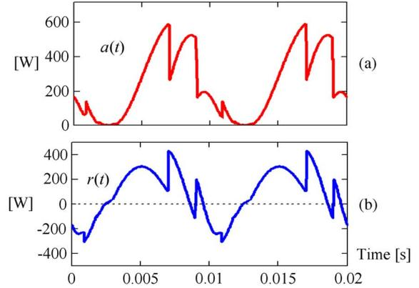
Fig. 18. Instantaneous active  $a(t)$  and reactive  $r(t)$  powers for the circuit of Fig. 15. (a) Active power. (b) Reactive power.
