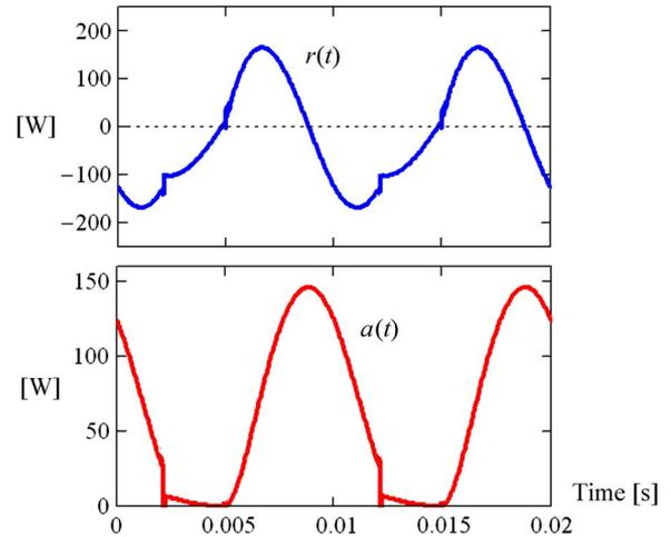
Fig. 22. Instantaneous reactive  $r(t)$  and active  $a(t)$  power components for the circuit of Fig. 19.
