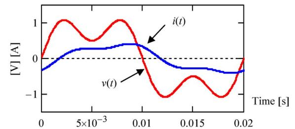
Fig. 23. Nonsinusoidal voltage excitation and corresponding current.
