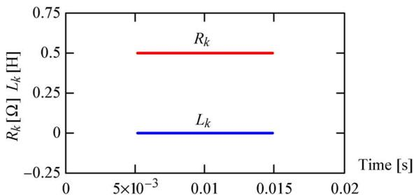
Fig. 10. Calculated results for the solution on (11) for a controlled rectifier feeding a resistive load.
