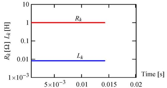
Fig. 13. Calculated results for the solution on equation (11) for a half-wave rectifier feeding an  $R-L$  load.
