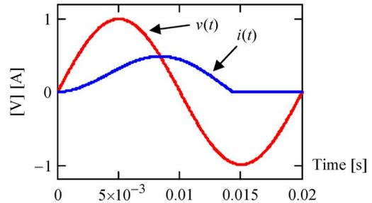
Fig. 12. Voltage and current for a half-wave rectifier feeding an  $R-L$  load.
