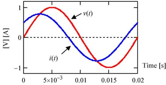
Fig. 26. Terminal voltage and current for the capacitive circuit.
