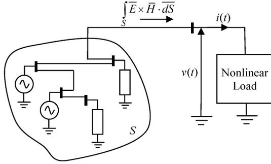
Fig. 1. Application of the Poynting theorem to a source and a nonlinear load.
