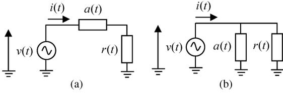
Fig. 2. Models for the representation of power phenomena in nonlinear circuits. (a) Series equivalent circuit. (b) Parallel equivalent circuit.
