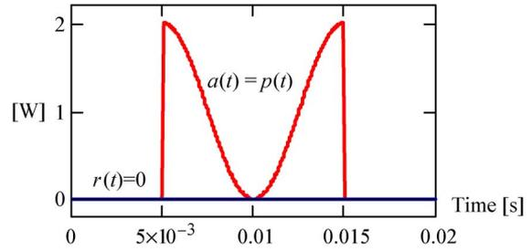
Fig. 11. Instantaneous active and reactive powers corresponding to the voltage and current signals of Fig. 9.
