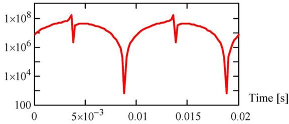
Fig. 7. Variation of the condition number with time for the family of matrices corresponding to Example A: Linear  $R-L$  circuit (signals of Fig. 4).
