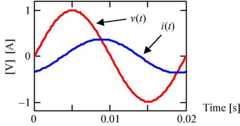
Fig. 4. Instantaneous current and voltage for a linear  $R$ - $L$  circuit.
