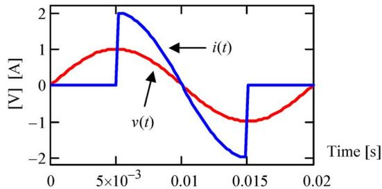
Fig. 9. Current and voltage for a controlled rectifier feeding a resistive load.
